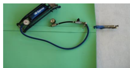
Pressure test of a double seam with an electronic pump
