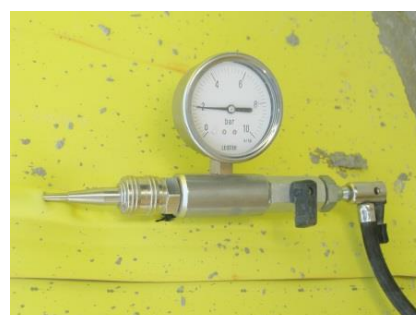
Pressure testing needle with manometer
