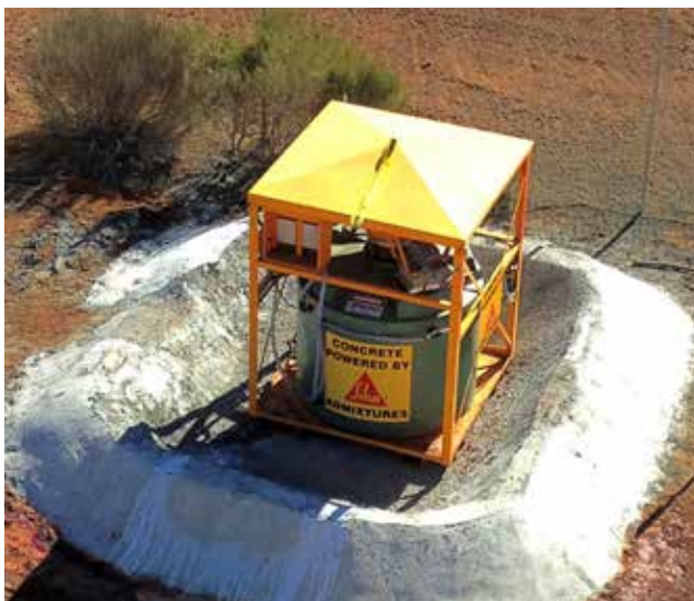
Figure 3: Simple site mixing equipment for producing liquid Sigunit® accelerator from instant Sigunit® powder
